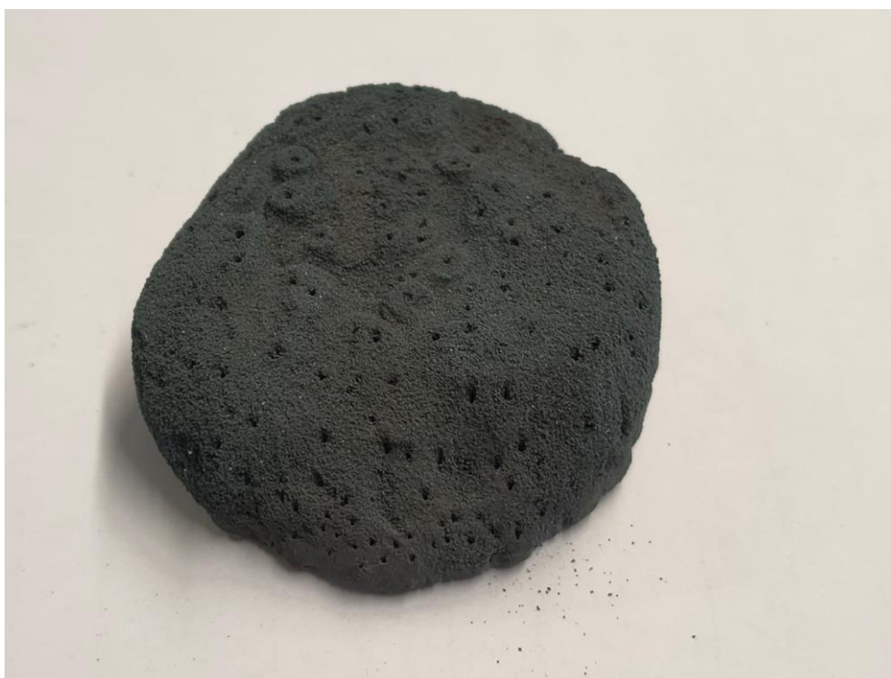
Figure 11 Agglomeration oxidation Feresint RI 250/2,1
