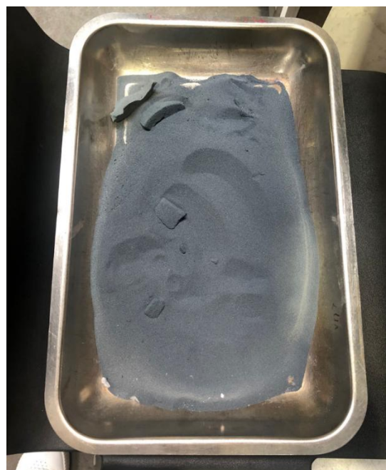
Figure 13b. Image of agglomerates extracted from the bed after inspection when operating at 700 °C and a bed height of 39 cm
