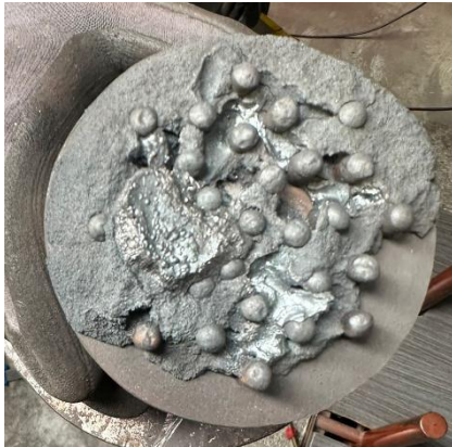
Figure 4a. Bell-type distributor plate with melting material.
