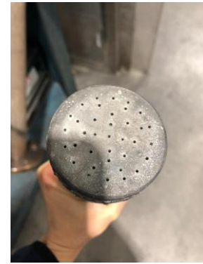
Figure 4c. New flat perforated plate for oxidation tests.
