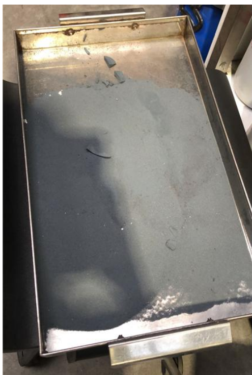
Figure 13a. Image of agglomerates extracted from the bed after inspection when operating at 750 °C and a bed height of 39 cm.
