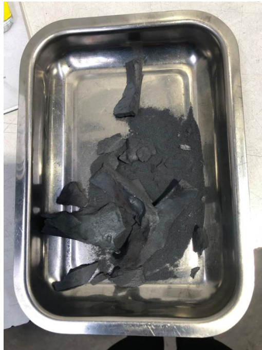
Figure 12. Image of agglomerates extracted from the bed after inspection when operating at 800 °C and a bed height of 39 cm.
